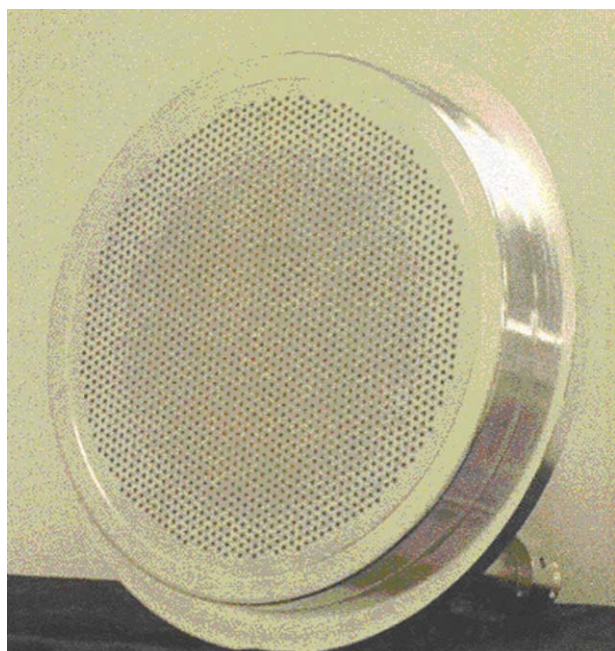
Figure 1 Plasma jet nozzle with many pores. [Color figure can be viewed in the online issue, which is available at wileyonlinelibrary.com .]
